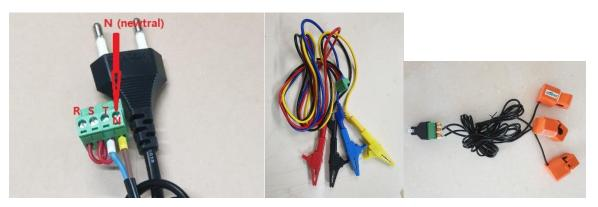
If you want to measure single phase with 3-channel display by using 3 current clamp, please make the cable connection as the above photo left.
