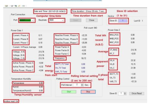
When starting the software, please check the "Port" number is correct or not. If it is okay, please press the "Open" button then you could see the 30 kinds of data at once with 2 seconds interval. If you are not satisfied, you can change from 2 seconds to 200 seconds.
